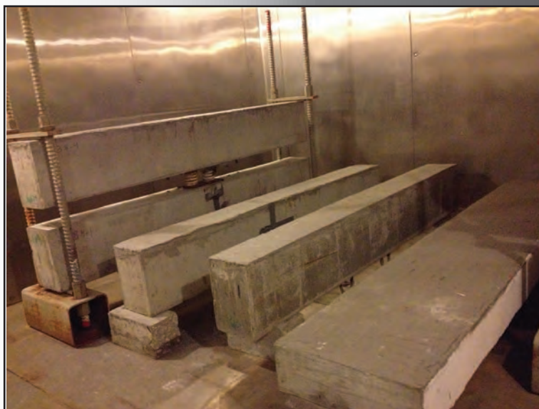
Figure 1. Beams inside Environmental Chamber
