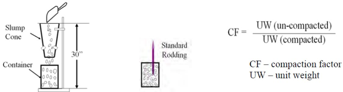
Figure 10. Compaction factor test setup [6].
