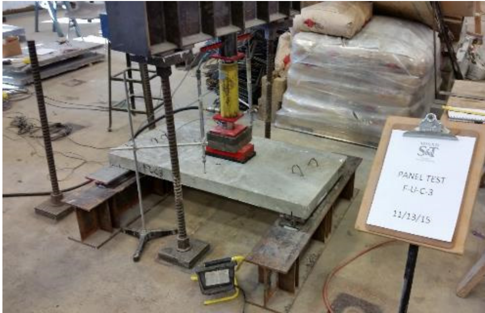
Figure 6.8. Panel FUC3 test setup
