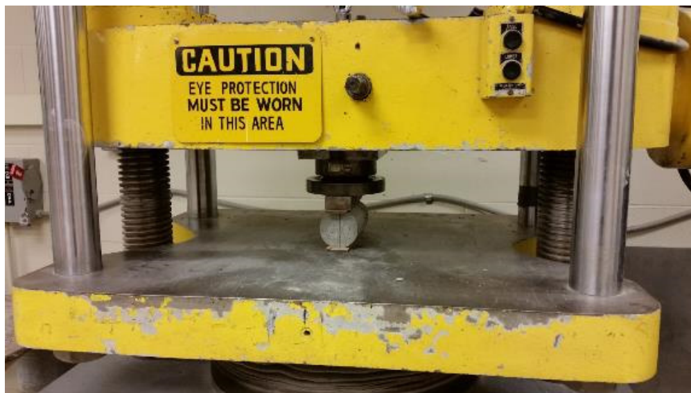
Figure 5.5. Split tensile strength test setup
