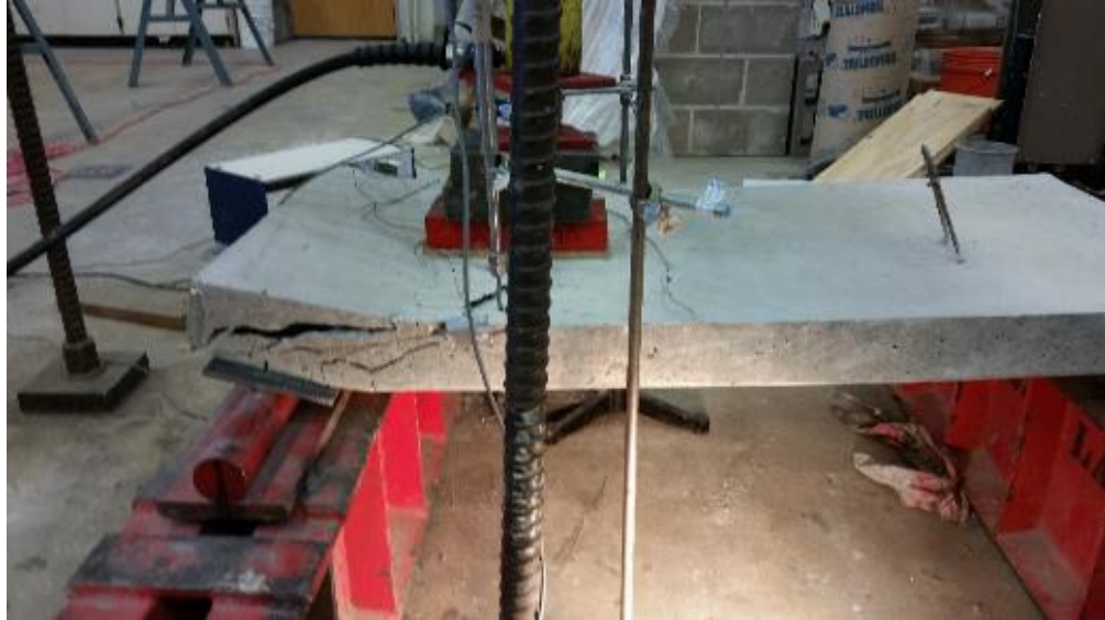
Figure 6.35. Diagonal tension failure on panel SCC3
