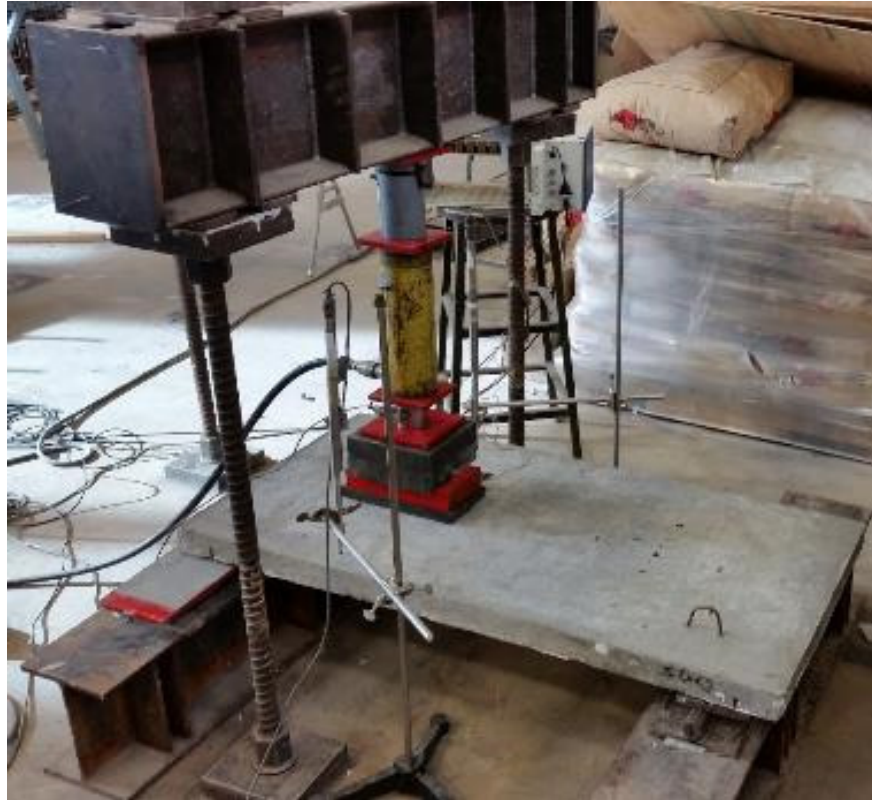
Figure 6.48. Panel SUC2 test setup
