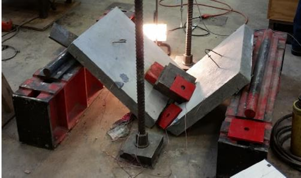
Figure 6.5. Panel FCW3 split after failure
