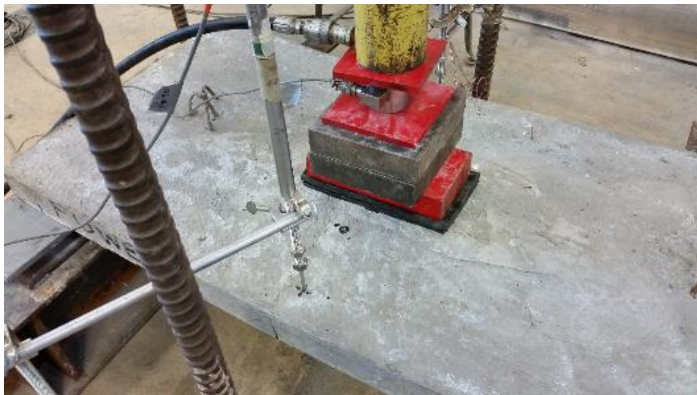
Figure 6.9. Panel FUC3 after failure
