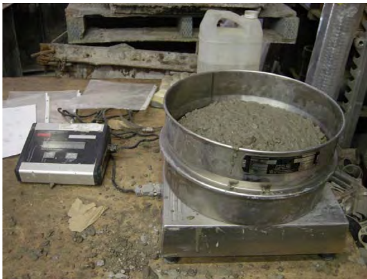
Figure 16. Sieve stability test.
