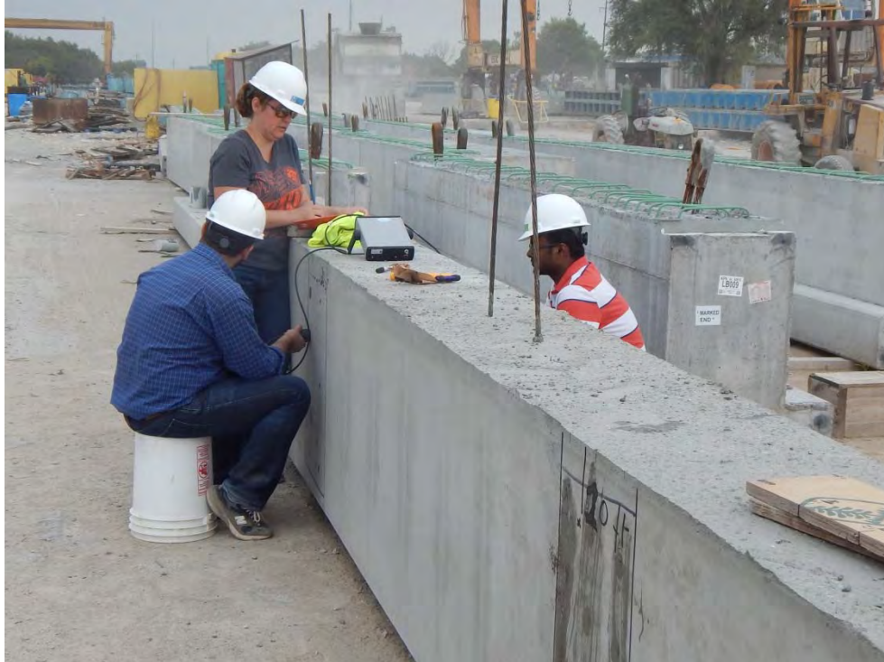
Figure 35. Dr. Hartell and her team performing the UPV measurements.
