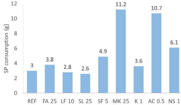
Figure 11. SP consumption of binary mixtures.
