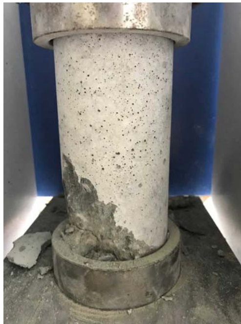
Figure 18. 2 day strength of mix SL-B-AC
