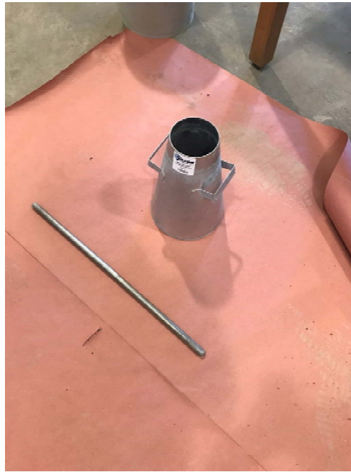
Figure 9. Slump test apparatus
