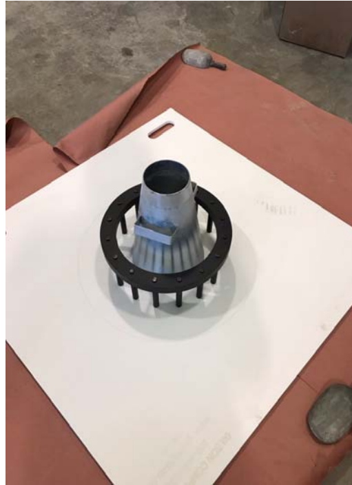
Figure 10. J-ring test apparatus
