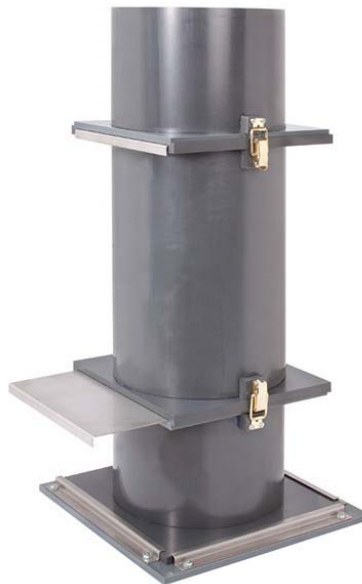
Figure 12. Column segregation test
