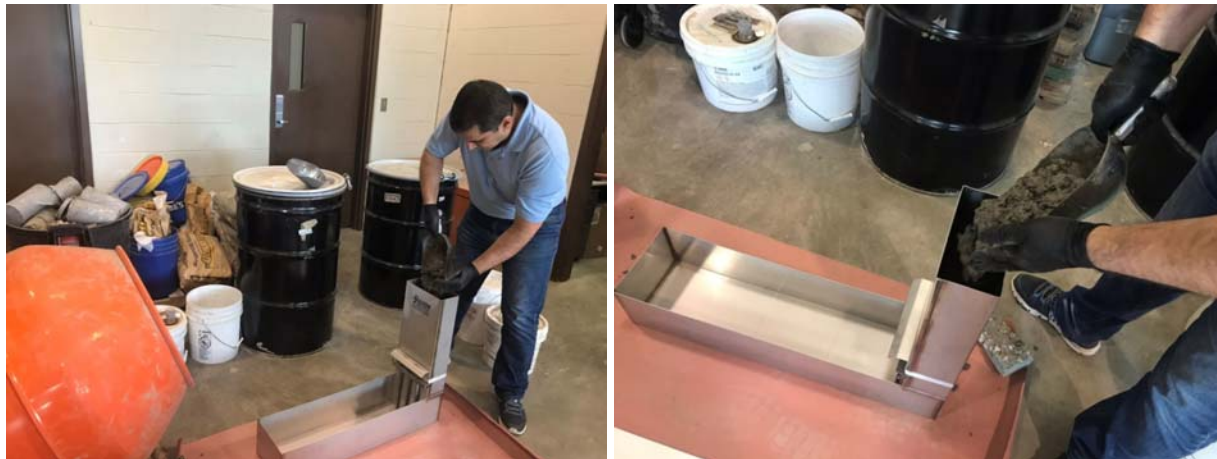
Figure 16. L Box test (Mixing design SL-B-AC)
