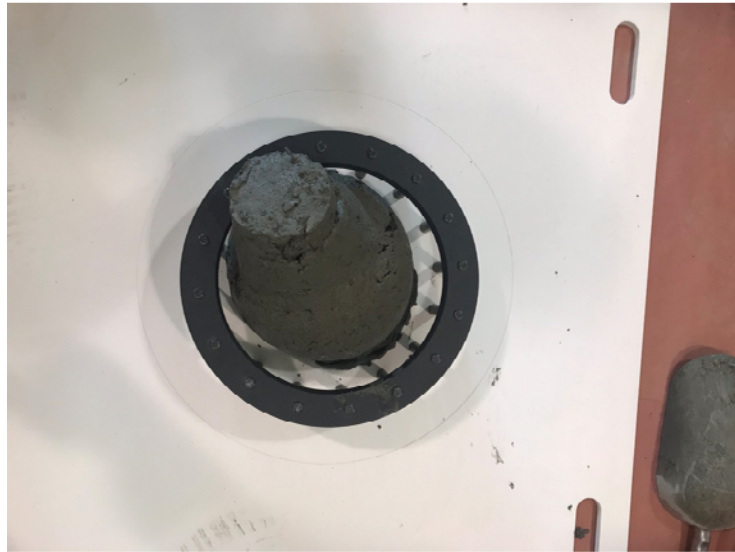
Figure 15. J ring test (Mixing design AC)
