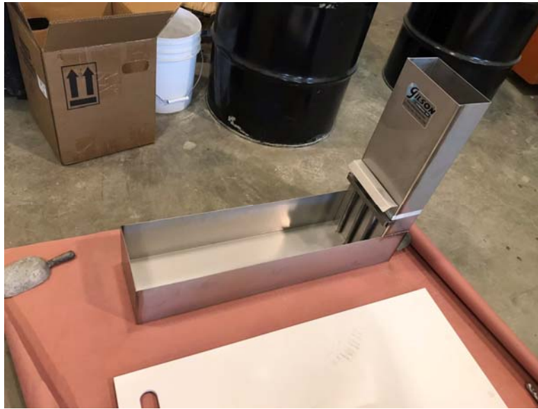
Figure 13. L box test
