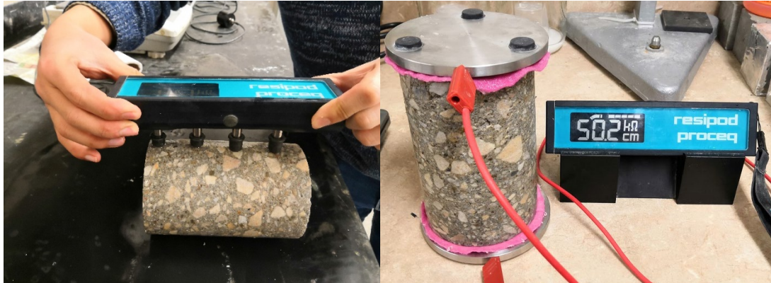
Figure 26 - Testing apparatus for surface resistivity (left) and bulk resistivity (right)
