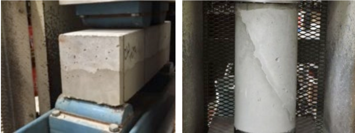
Figure 4.1: Composite Prism Test Specimen (l) and Slant Shear Test Specimen (r)
