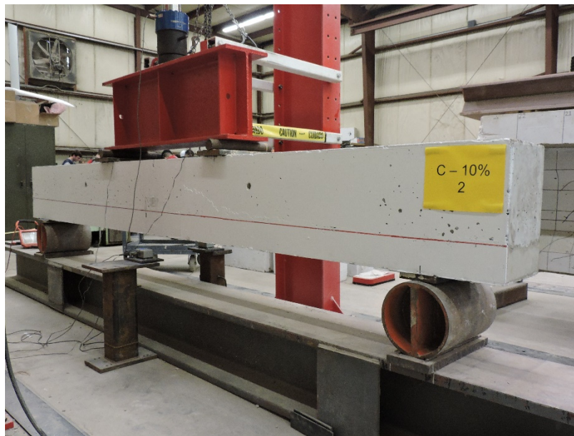
Figure 5.14: Photograph of Full-Scale Beam Specimen Test Setup
