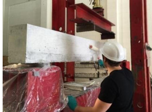
(b) Painting beams for flexural testing
