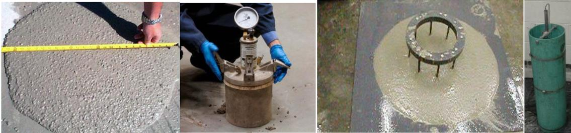
**Figure 3-1: Testing fresh properties**
