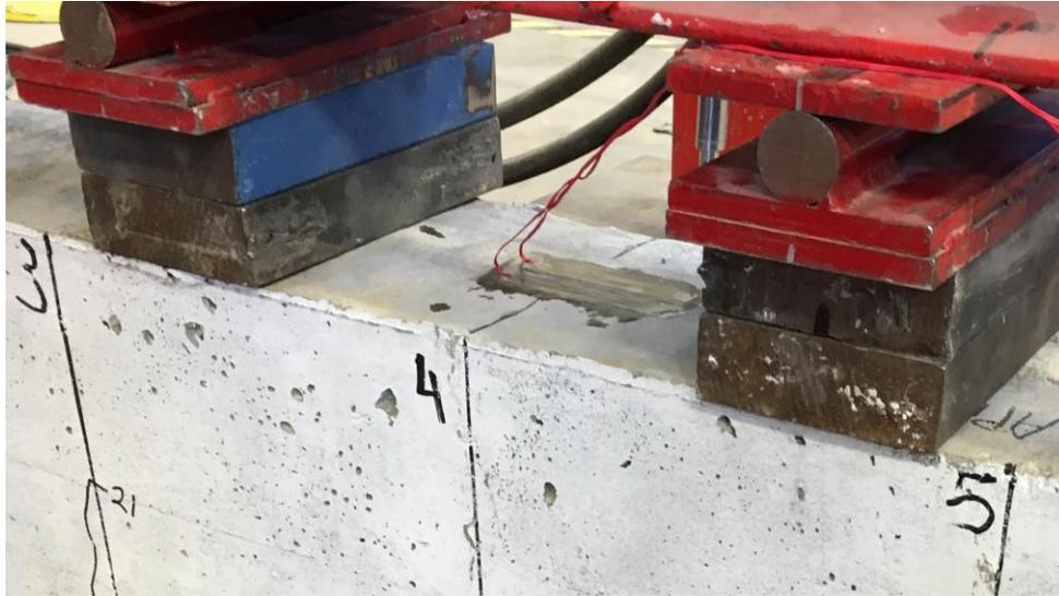
**Figure 5-4: Concrete surface attached strain gages**
