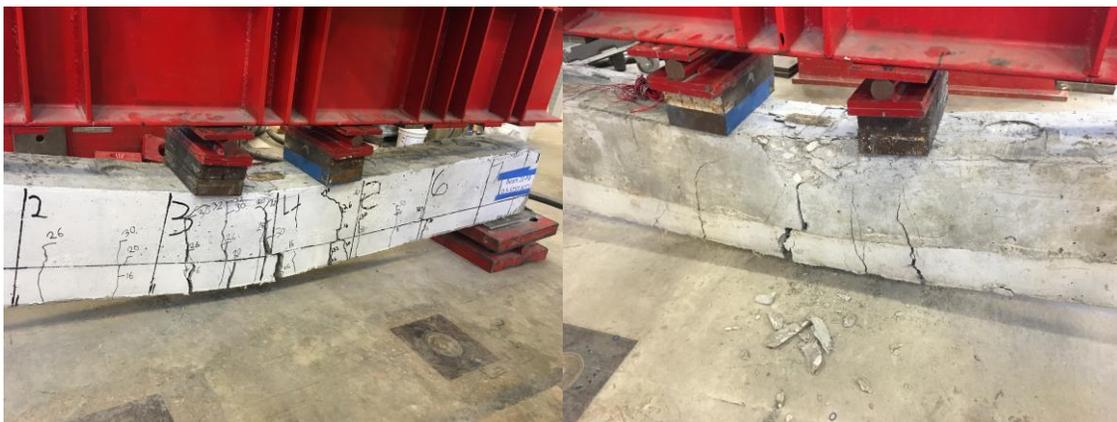
**Figure 5-13: Testing of Repaired beams**
