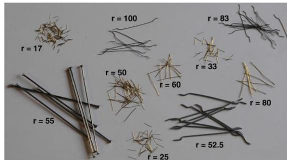
**Figure 2-28: Different fibers tested [37]**
