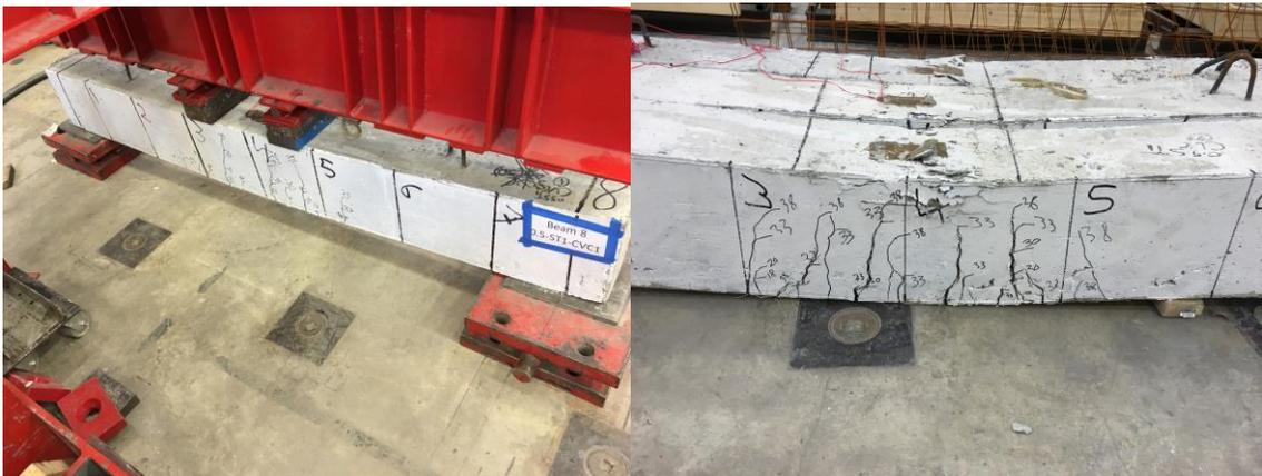
**Figure 5-12: Testing of monolithic beams**
