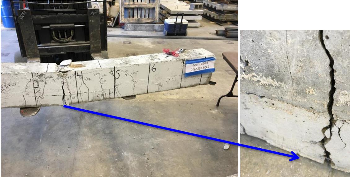
**Figure 5-19: Repaired beam after loading up to failure**
