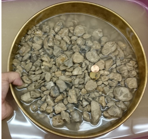
Figure 7-1. Washing of RCA Samples
