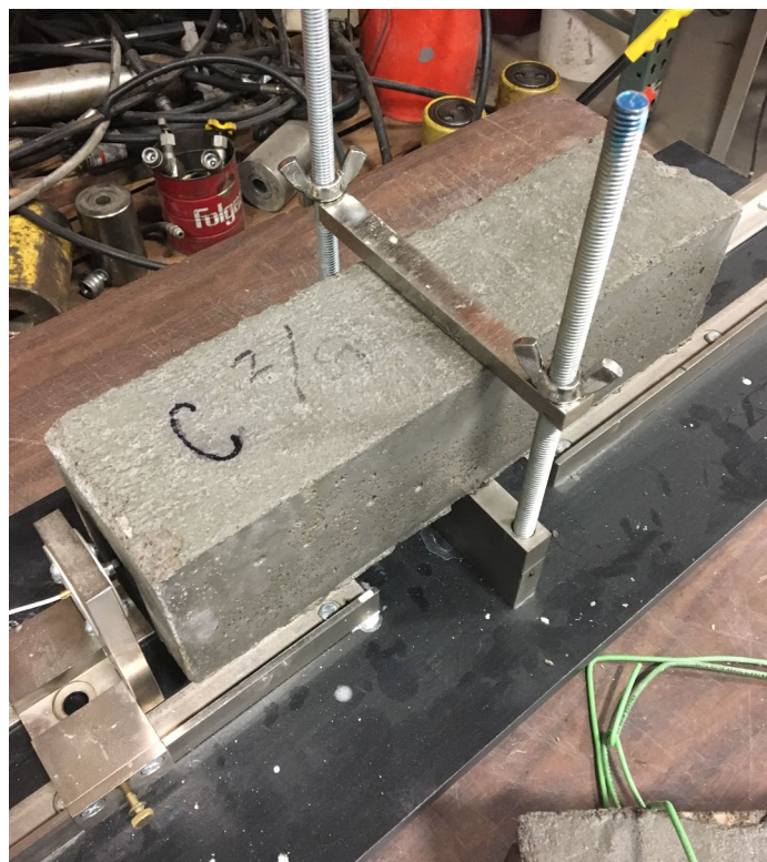
Figure 9-2. Longitudinal Dynamic Modulus of Elasticity Test Setup
