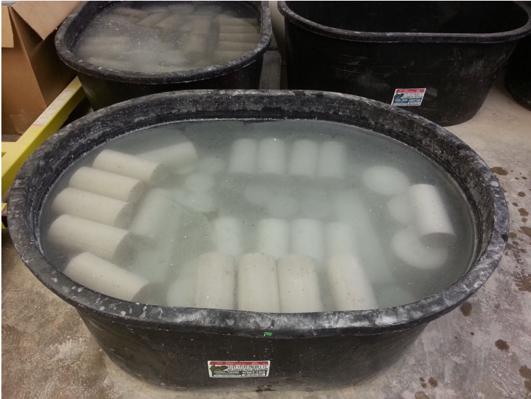
Figure 9-3. Constant Temperature Lime Water Tempering Tank
