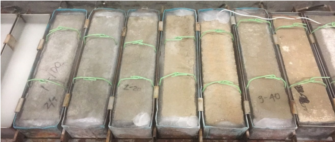
Figure 5-1. Freeze/Thaw Specimens within Test Chamber
