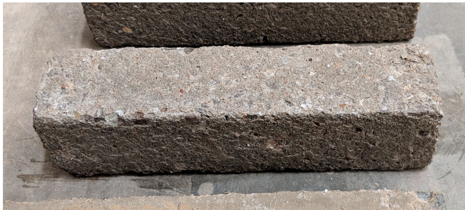
Figure 9-7. Mix 2-20 Specimen at 304 Freeze/Thaw Cycles
