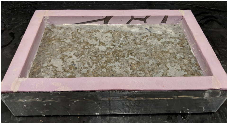
Figure 9-13. Mix 3-60 Salt Scaling Specimen at 50 Cycles
