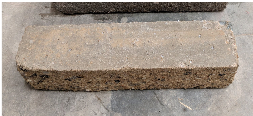
Figure 9-8. Mix 2-60 Specimen at 304 Freeze/Thaw Cycles
