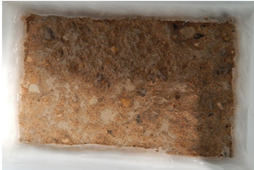
Figure 6-16. 25 Percent RCA Specimen After 15 Cycles
