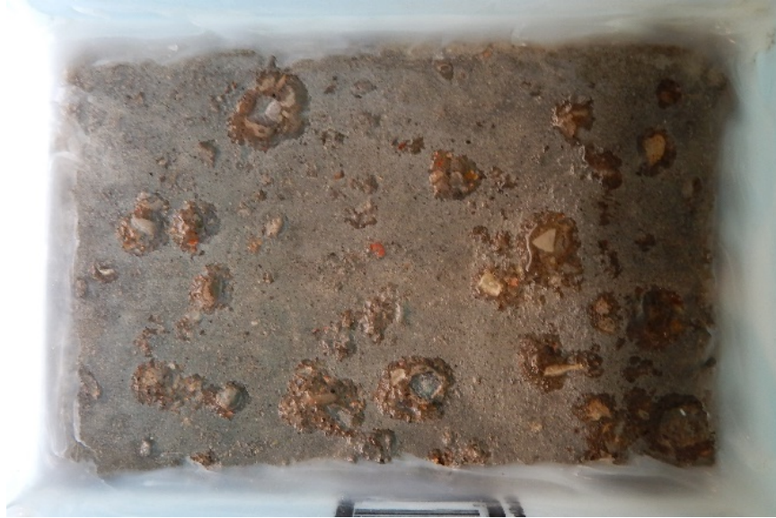
Figure 6-19. 100 Percent RCA Specimen After 50 Cycles
