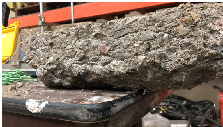
Figure 5-8. Control Mix Specimen at 304 Freeze/Thaw Cycles
