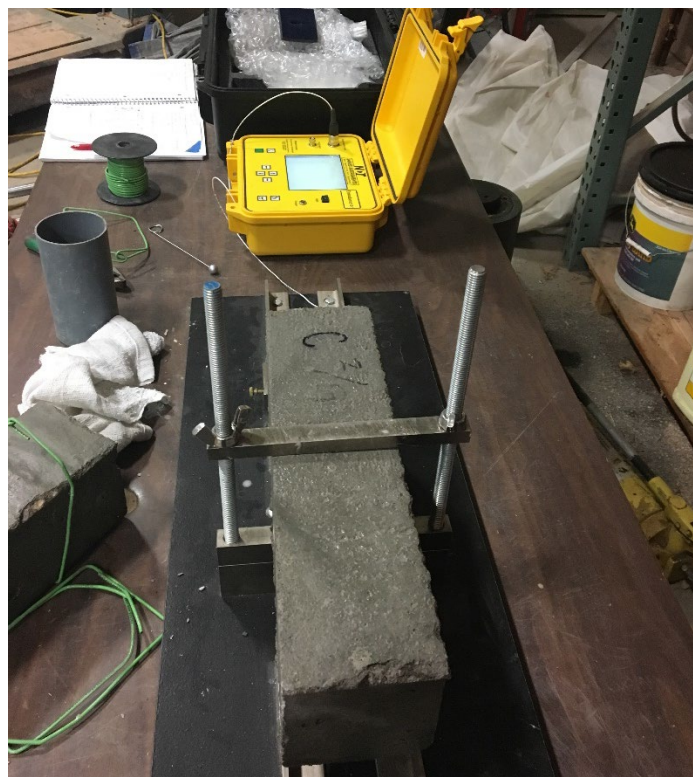
Figure 5-2. Longitudinal Dynamic Modulus of Elasticity Test Setup
