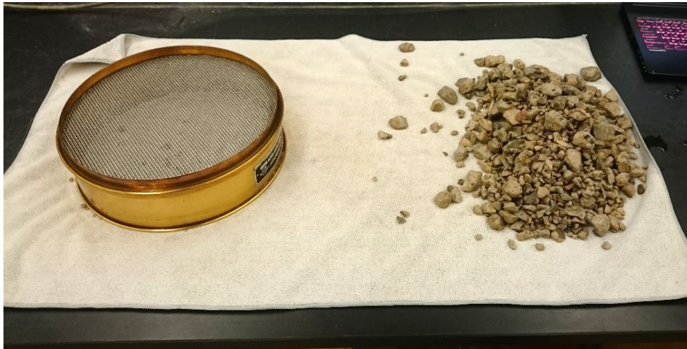
Figure 7-2. Aggregate Preparation for Moisture Measurements
