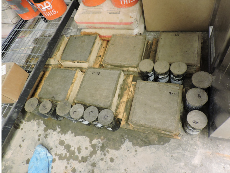
Figure 5-4. Salt Scaling Specimens as Cast
