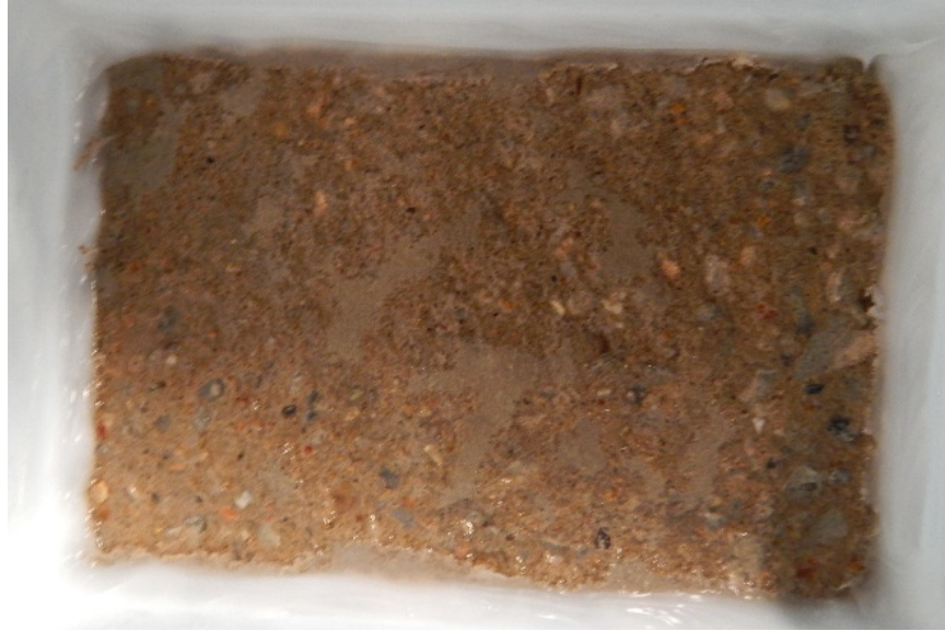
Figure 6-21. 40 Percent Fly Ash Plus 100 Percent RCA After 35 Cycles
