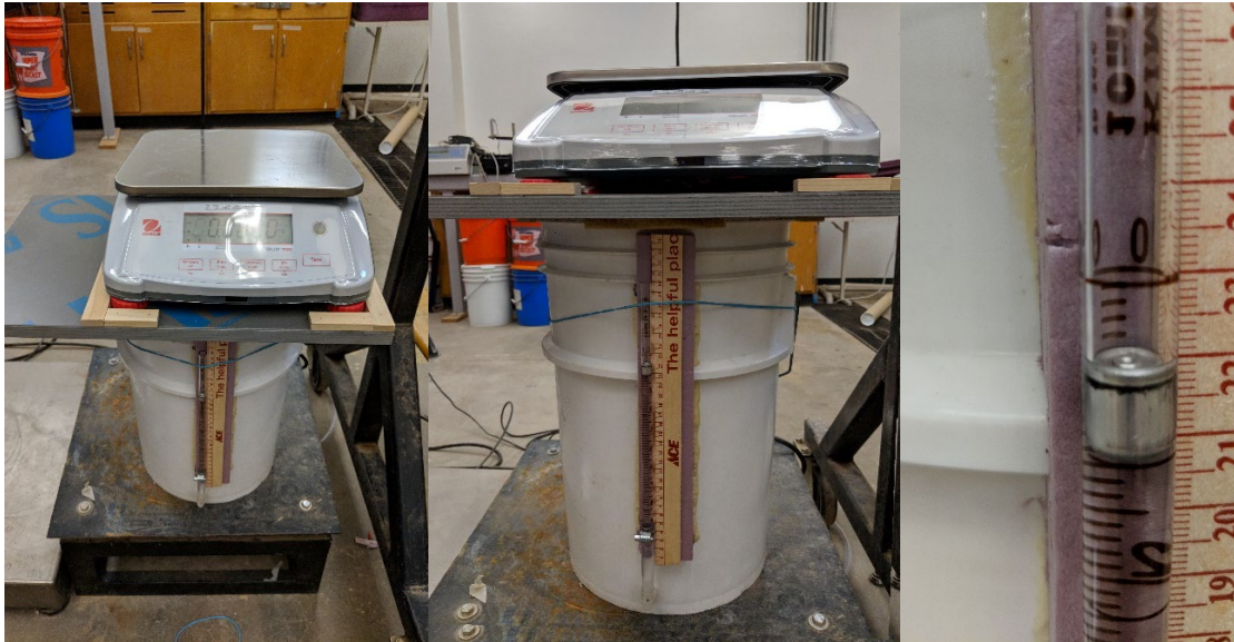
Figure 7-8. Hydrostatic Weighing Setup
