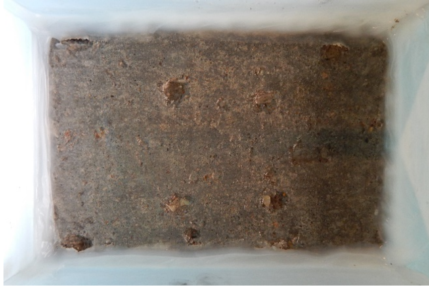
Figure 6-17. 50 Percent RCA Specimen After 50 Cycles
