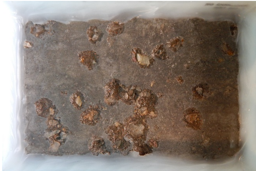
Figure 6-18. 75 Percent RCA Specimen After 50 Cycles
