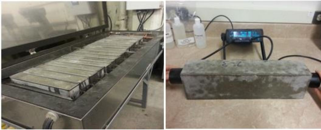
Figure 39- Freezing and thawing cabinet (left); measurement of pulse velocity (right)
