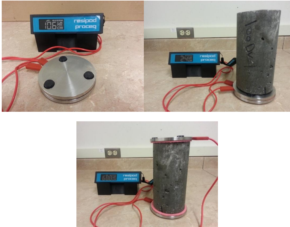
Figure 35- Measuring bulk electrical resistivity
