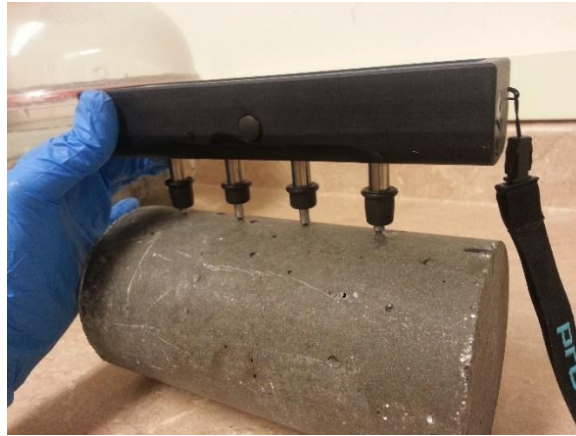
Figure 34- Surface resistivity measurement
