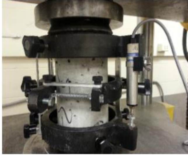
Figure 28- Modulus of elasticity test setup
