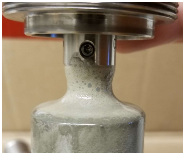
Figure 169. The pressurization/depressurization of the samples yielded a substantial volume of foam on top of the inner cylinder of the pressure cell. Picture taken after removing the inner cylinder from the pressure cell.
