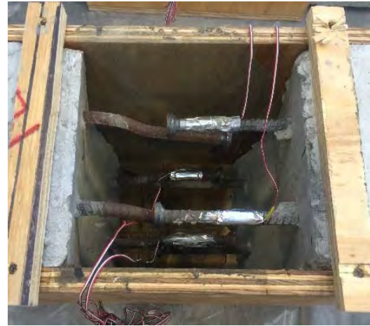
Figure 3.6 Anchored rebar detail
