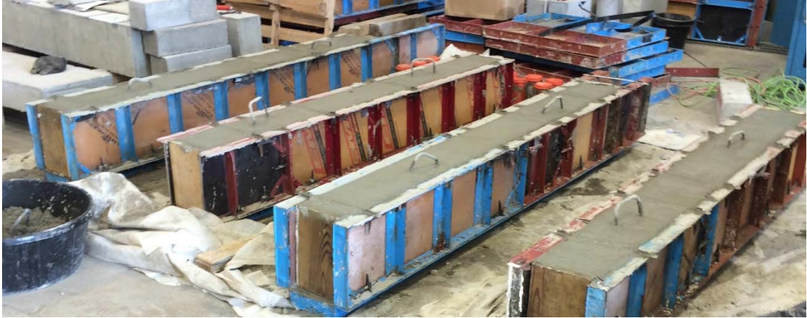
Figure 5.2 Control specimens after casting
