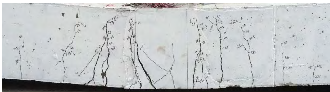
(c) UHSC specimen B-18-U-R-S at failure Figure 6.22 Specimens at failure (cont.)
