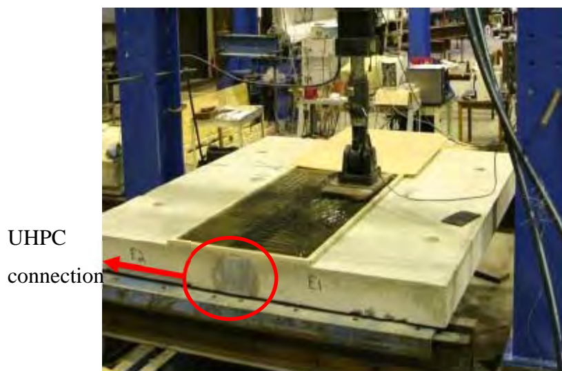
Figure 2.5 Test setup used in FHWA study HRT-11-023
