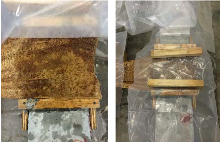
Figure 5.20 Curing using burlap
