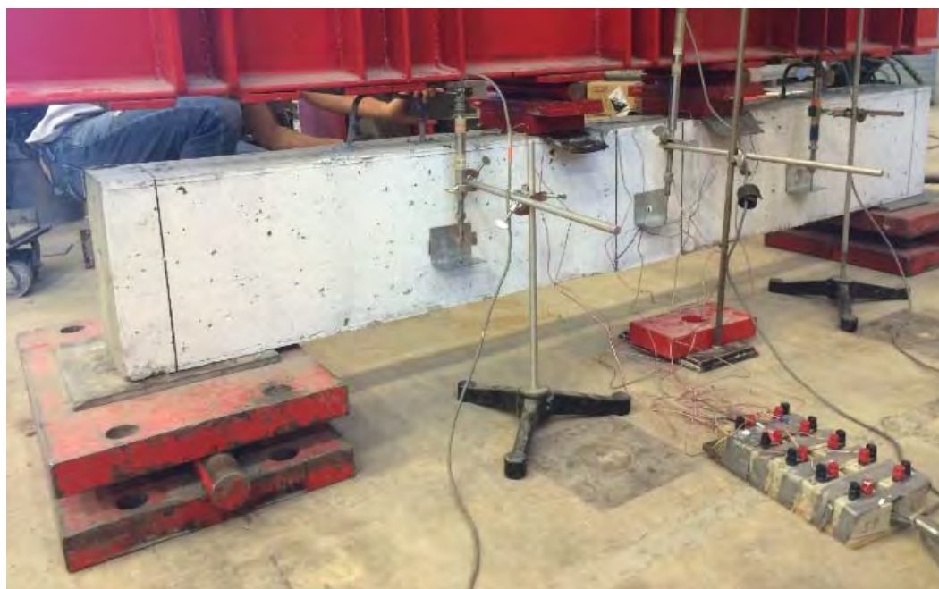
Figure A. 2 Location of LVDTs
