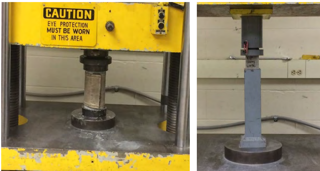
Figure 5.17 Testing cylinder and cube in Tinius Olsen
