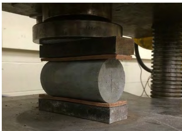
Figure 5.18 Splitting tensile test on UHSC specimen
