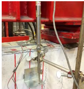
Figure 5.9 LVDT at midspan
