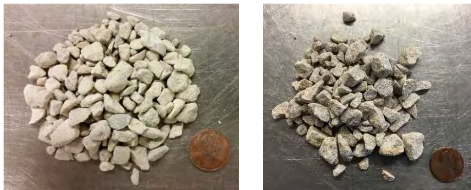
Figure 4.3 Coarse aggregate (a) 1-in. limestone (b) 3/8-in. crushed limestone
