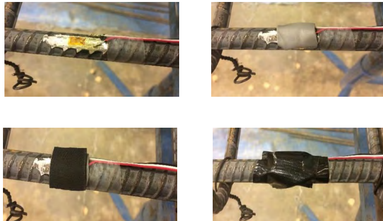
Figure 5.10 Strain gauge installation
