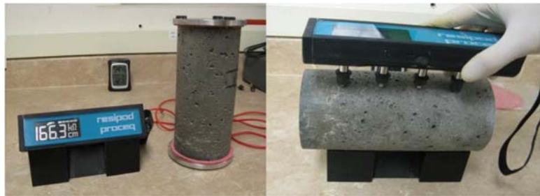
Figure 3.6: Bulk electrical conductivity (left) and surface resistivity (right)
