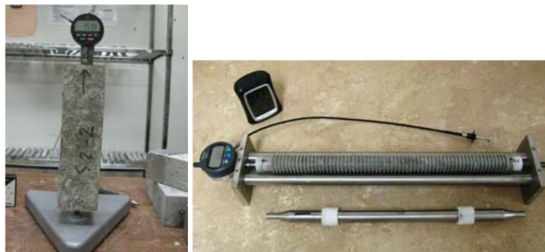
Figure 3.5: Drying shrinkage (left) and autogenous shrinkage (right)
