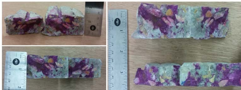
Figure 10: Carbonation depth measurement of the concrete cores
