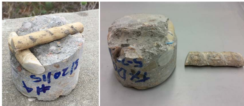
Figure 7: GFRP extraction from the concrete cores
