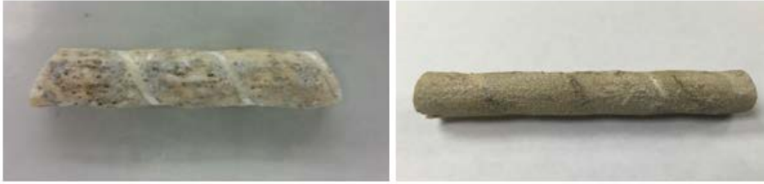
Figure 19: No. 6 (left) and No. 5 (right) GFRP bars tested for horizontal shear strength
