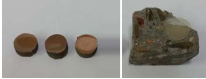
Figure 8: Prepared samples prior to SEM analysis: GFRP (left) and concrete-GFRP (right)
