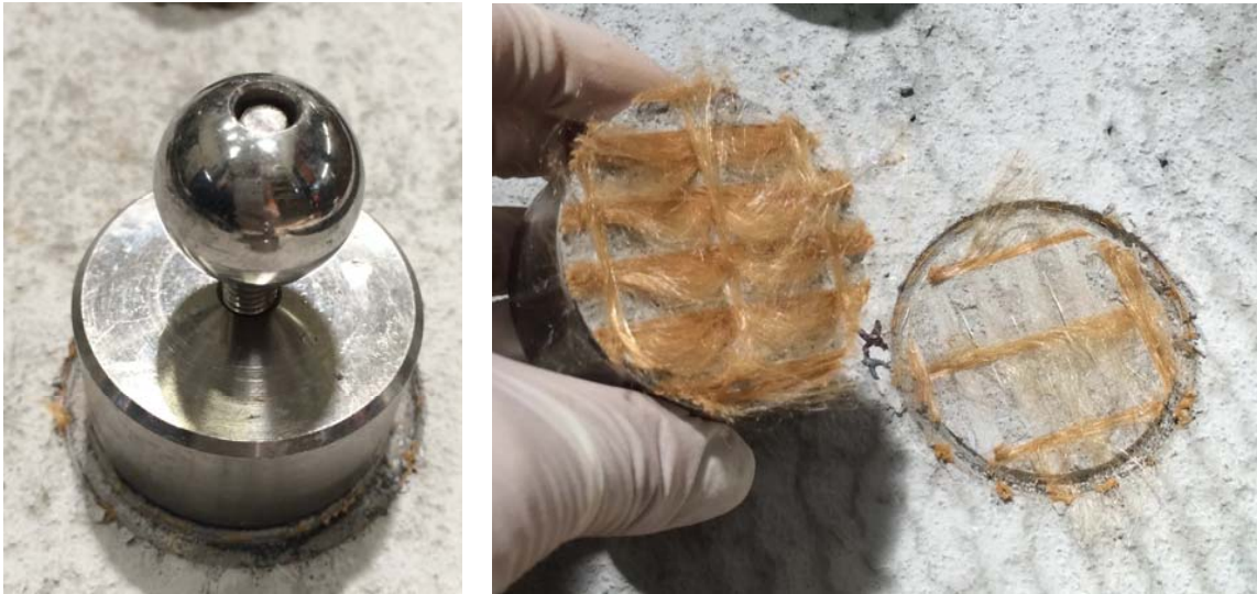
Figure 2-22 –Bond Strength Over Repair Mortar Primary Failure Mode
