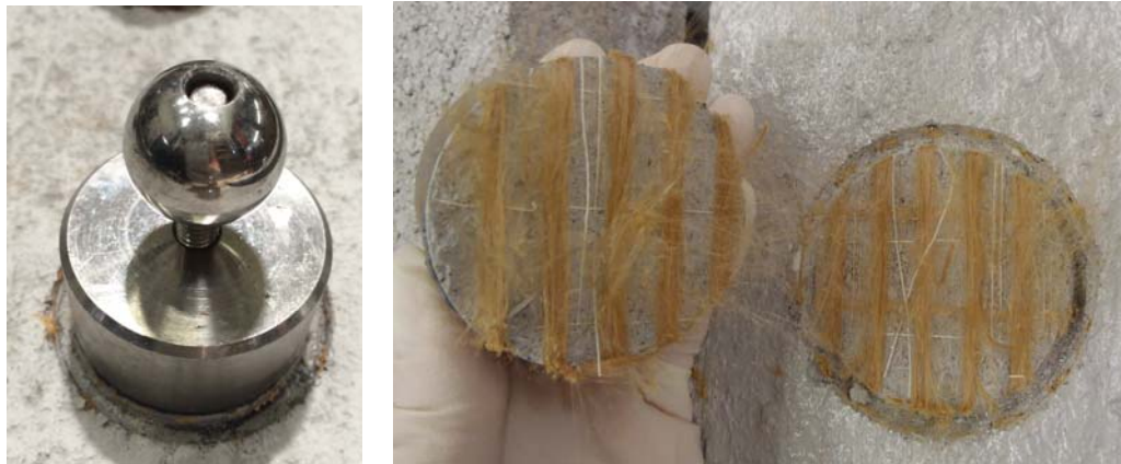
Figure 2-25 – Bond Strength Over Repair Mortar Primary Failure Mode
