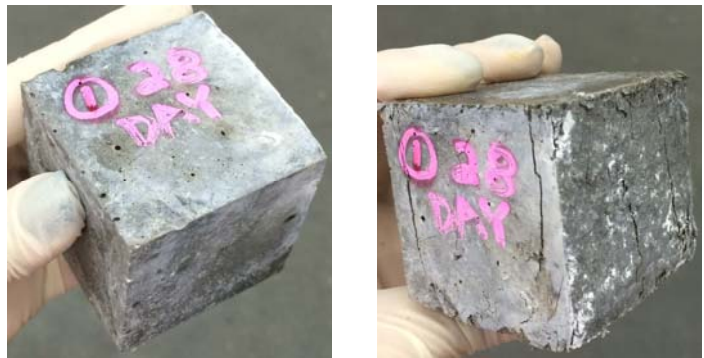
Figure 2-7 –Repair Mortar Cube Failure Mode
