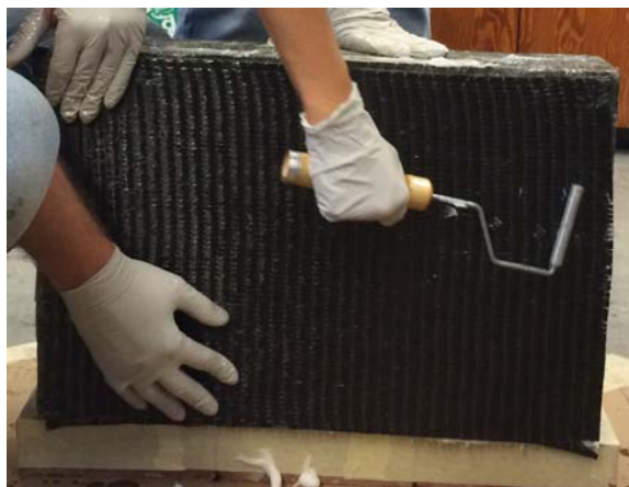
Figure 3-6 – FRP Application to Concrete Specimens
