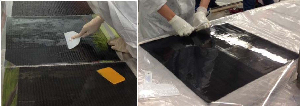
Figure 3-4 – FRP Panel Fabrication
