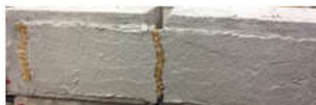
Fig. 5. Bending test results: (a) Bending test strength with respect to the exposure, (b) Slippage in the PBO-FRCM composite for one ply, and (c) Debonding of FRCM composite for four plies
