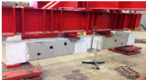
Fig. 4. Beam test set-up
